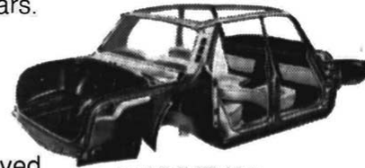
Rover's Welded Steel Cage
